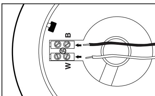
4 Secure wires by tightening terminal screws into wires with small flat-head screwdriver.
