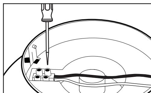
5 Connect fixture wires to junction box wires using provided wire nuts. (Black line voltage, White neutral)
