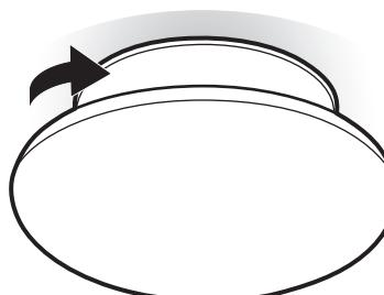
Motion Sensor will turn fixture on when motion is detected up to 9 feet away from fixture. Fixture will turn off after 10 minutes if no motion is detected. Sensitivity of motion sensor will be affected by obstructions such as walls, doors, etc. Relocate the fixture to a different socket if obstruction prohibits operation of the sensor.
