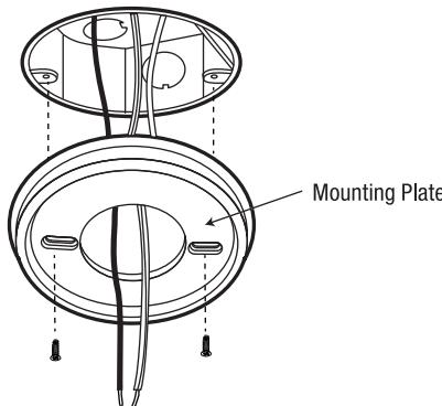
3 Insert provided wires into fixture terminal. Insert black wire into B slot. White wire into W slot.
