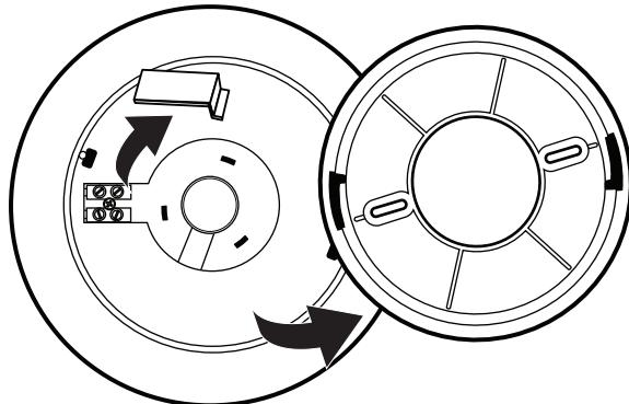
2 Install mounting plate to junction box, using provided screws. Make sure side labeled "faces ceiling" faces the ceiling.
