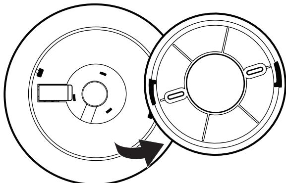
**2** Remove cap to expose screw base.
