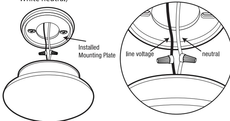
6 Line up pin guides on fixture to notches on mounting bracket and twist fixture clock-wise until it locks into place.
