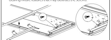
4 Install side brackets between fixture and grid, making sure to insert tabs of side brackets into slots of end brackets.
