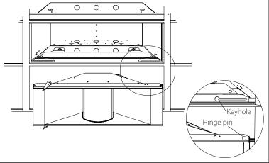
6 Hook the safety cables into the holes located on the end brackets. Connect wiring as shown. Grey and purple wiring are for 0-10V dimming systems. Cap off if not used.
