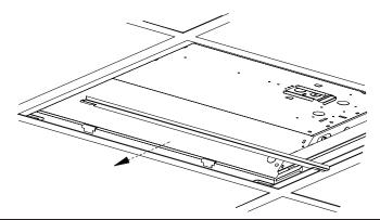
5 Insert hinge pin of the TAR main body into the keyholes of the end bracket, then slide to the end of the slots.
