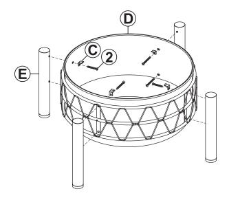
Align one Leg (E) with the outside of Fire Bowl (D). Secure the bottom mounting hole using one M6x30mm Bolt (2). Then, align Bracket (C) with the top mounting hole and secure using one M6x30mm Bolt (2).
