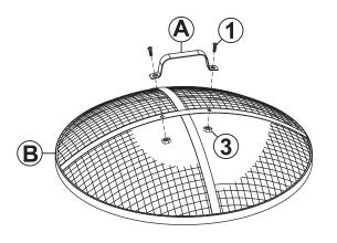
Fasten Handle (A) to Spark Screen (B) using two M6x12mm Bolts (1) and two Nuts (3).
