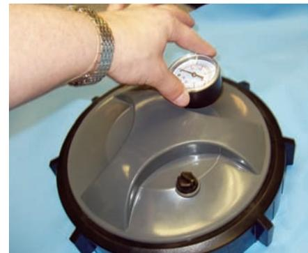
Figure 25b — Installing pressure gauge
