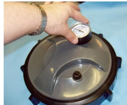
Figure 25b — Installing pressure gauge
