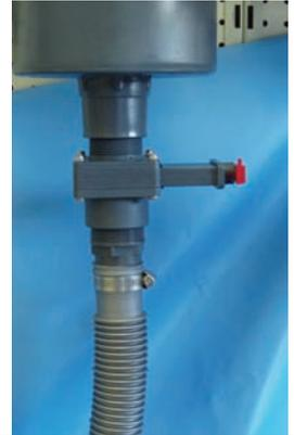
Figure 24 — Slide valve in closed position
