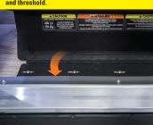
Two safety latches on either side of SolidStep securely locks it to the RV entry door frame.
