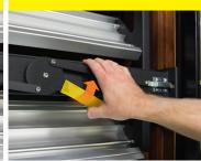
While holding the handle, release the SolidStep from the doorjamb. Slowly lower the step with both hands firmly supporting SolidStep.
