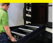
For uneven ground surfaces, remove pin on the extendible legs to adjust leg length.
