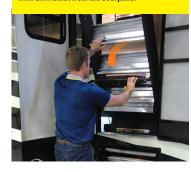
The Lift Assist strut keeps the SolidStep from dropping completely when disengaged from the door-jamb and will even support its own weight.
