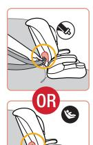
Locate Forward-Facing Belt Path & Route Vehicle Belt or Lower Anchor Belt Through It
