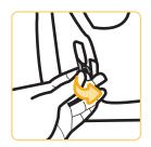
Undo Tab and Remove arm rest covers
