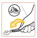
Loosely Attach Tether Hook to Vehicle's Top Tether Anchor
