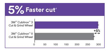
4. Results are based on an automated beveling of 1018 carbon steel bars. Cutting & grinding wheel geometry was 115mm outer diameter mounted on a servo motor with an applied force of 12 lbs. Cut speed is defined by metal removed after 10 minutes of testing. The total material removal is estimated based on the amount of wheel used for 10 minutes of testing life. End of life is assumed to be 50% of the initial wheel mass.
