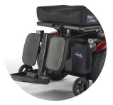
After the drive wheel climbs the curb, the chassis returns to level and the rear springs return to an uncompressed position.
