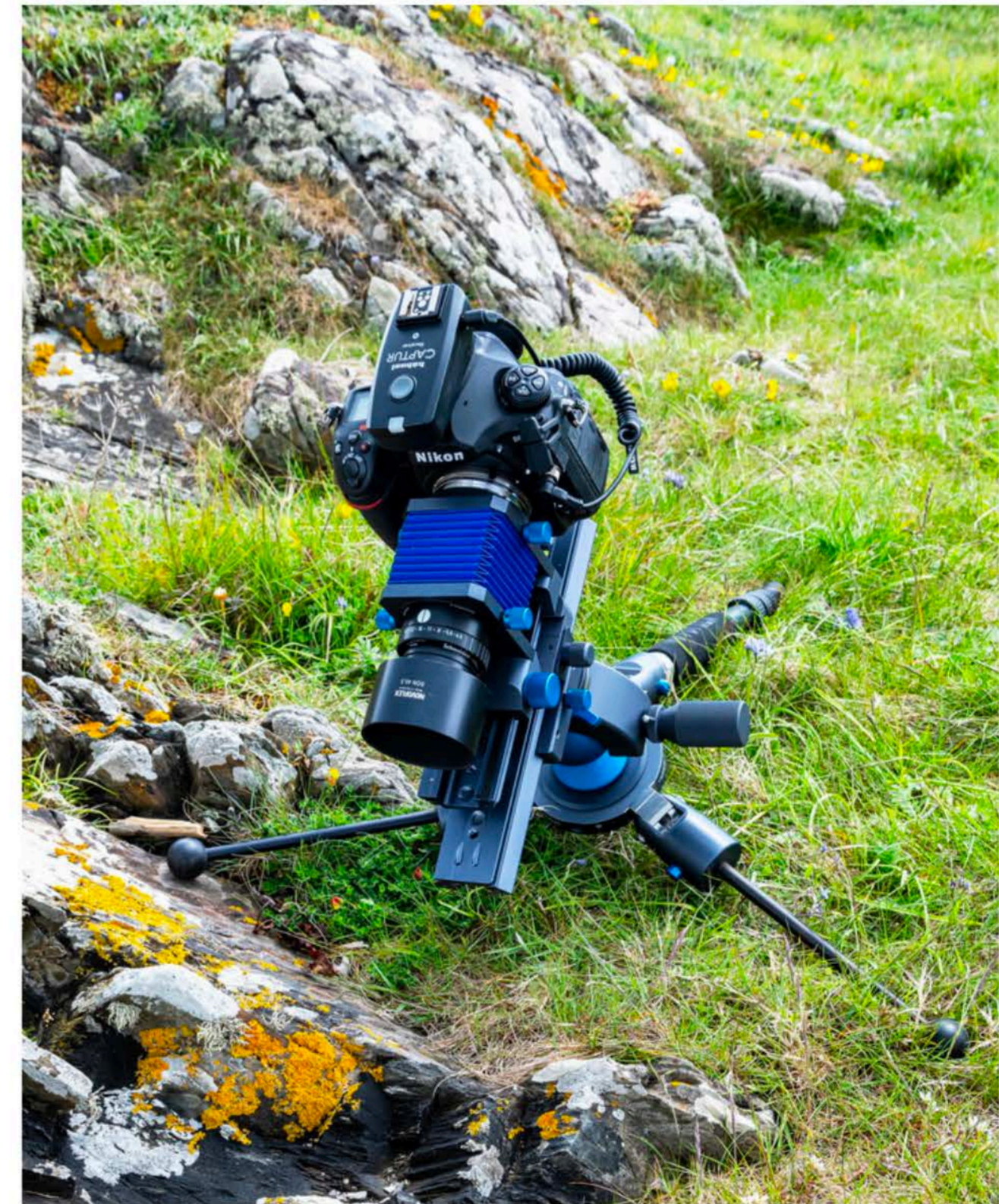
Photographing lichens using the BAL-F with the Castel XQ II focusing rail, the Schneider APO-Digital lens on the Nikon D850.
