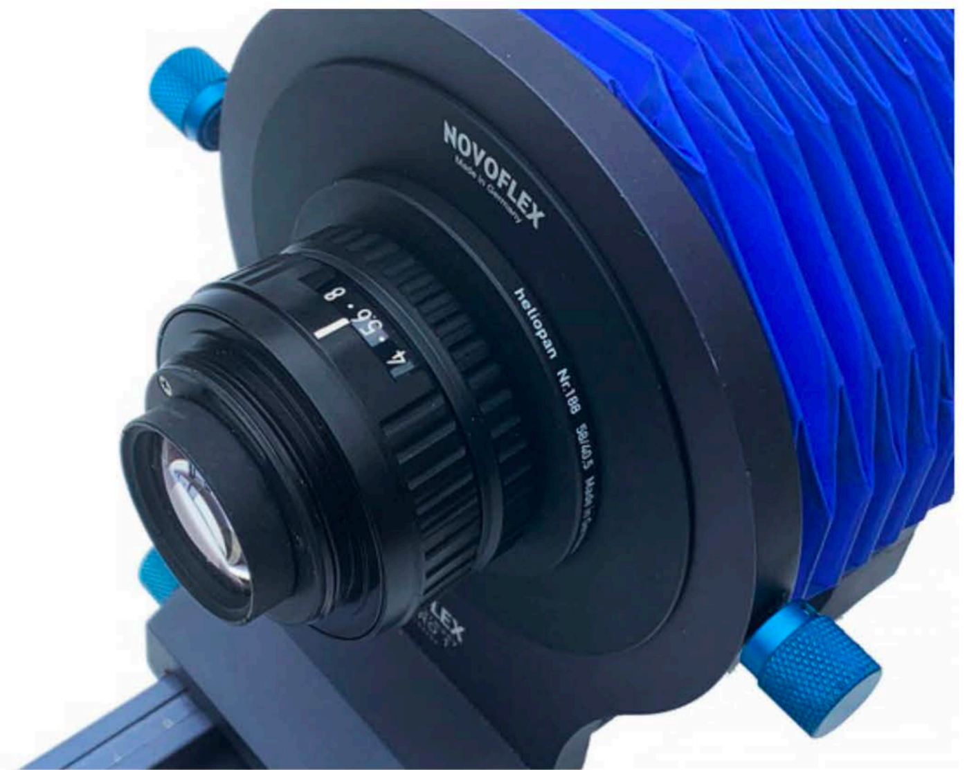
The EL-Nikkor 50mm enlarging lens on the BALPRO-1. This lens can also be used on the smaller BAL-F bellows. Magnifications in the region of 4X can be achieved with either bellows setup,
