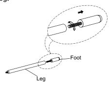
Step 3 Attach the Bottom Shelf and the Foot to the assembled base.
