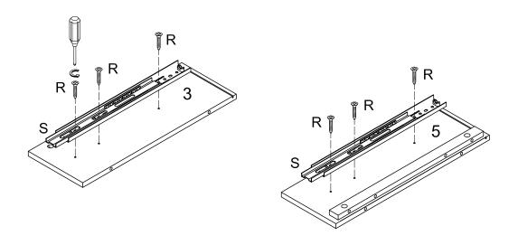
Secure slider arm (S) to side panel (3,5) with screw (R).
