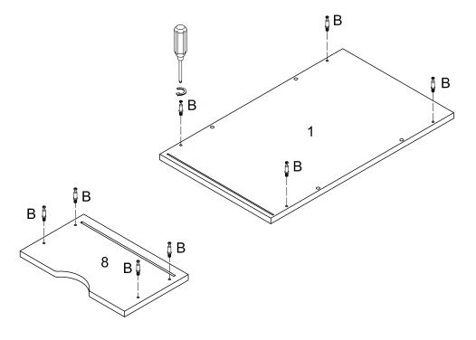
Secure cam bolt (B) to drawer front panel (8) and top panel (1).
