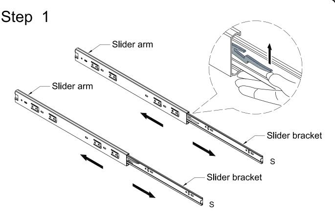
Disassemble drawer slider (S) by sliding the slider arm and slider bracket apart. Depress the small lever of the slider bracket and carefully pull the two pieces apart. Repeat this process for both drawer sliders (S).
