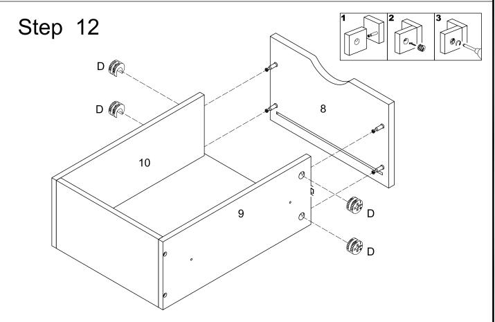
Insert drawer front panel (8) into drawer side panel (9,10), then insert and secure cam lock (D) to drawer side panel (9,10) to lock it.
