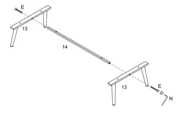
Use wrench (N) to secure leg (13) to part (14) with bolt (E).
