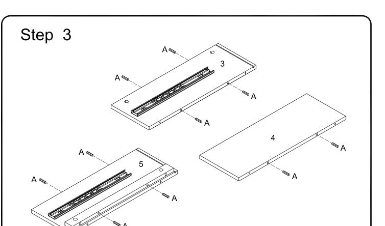
Insert wooden dowel (A) into side panel (3,4,5).
