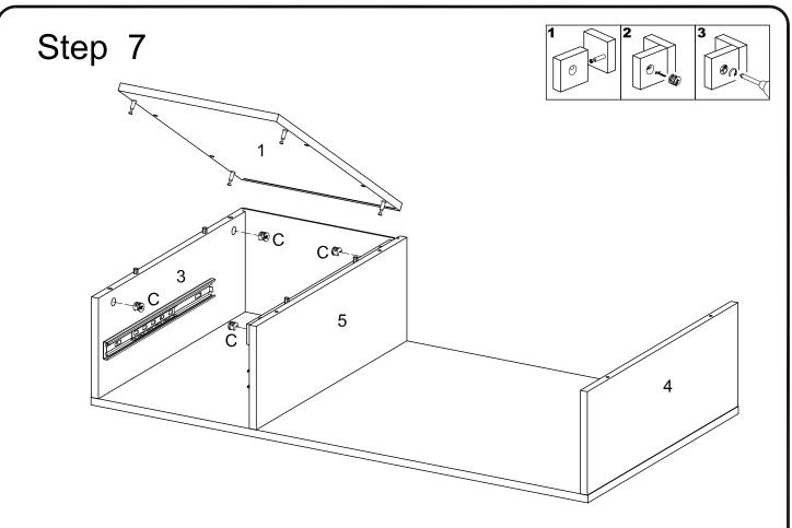
Insert top panel (1) into side panel (3,5), then insert and secure cam lock (C) to side panel (3,5) to lock it.
