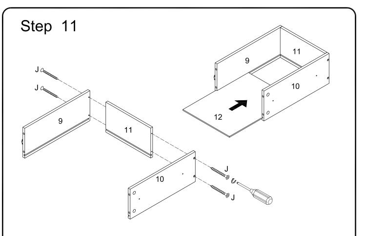
Secure drawer side panel (9,10) to drawer back panel (11) with screw (J), then slide drawer bottom panel (12) into grooves as per diagram.
