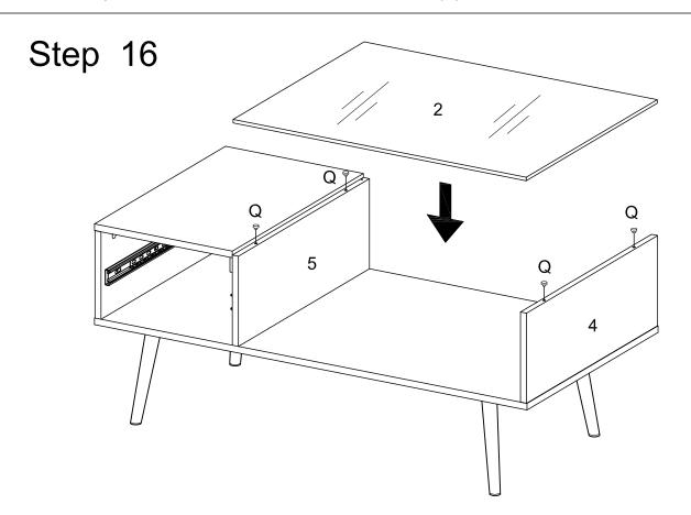
Place rubber suction cup (Q) over holes as per diagram, then place glass top on top of frame carefully.
