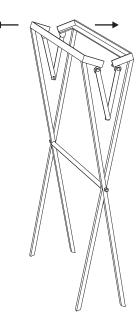
Step 1 Base -Using the long sides of the top of the base, push open until the hinges on each end are tight.
