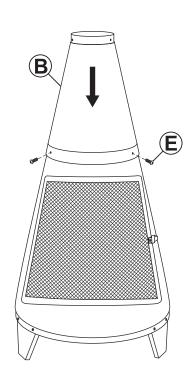
Flip unit upright and place Flue Base (B) onto the main body. Align the mounting holes and secure using three Bolts (E).
