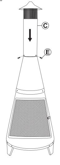
Place Flue (C) onto the flue base and firmly secure using three Bolts (E).
