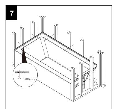
Drill 3/16" clearance holes in flat area of top flanges, and centered on each stud. Evenly space holes on front vertical flanges.
