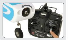
**27** Open the battery hatch, unplug the Li-Po battery and switch OFF the transmitter. Assemble the propeller and spinner in the following sequence:
