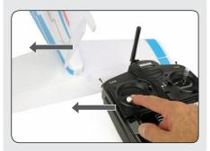
Make sure the control surfaces 22 operate in the correct direction. With the model in front of you, facing away, move the rudder stick to the left and check that the rudder moves left in response. Right rudder stick will move the rudder to the right.
