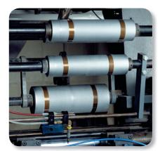
Conformable and self lubricating, 3M™ PTFE Tape 5480 helps the movement of web materials in many types of roller wrapping applications.
