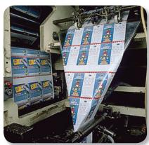
$3M^{^{\intercal}}$  UHMW-PE Tape 5423 is placed on a web former edge to minimise web friction as the web is folded.
