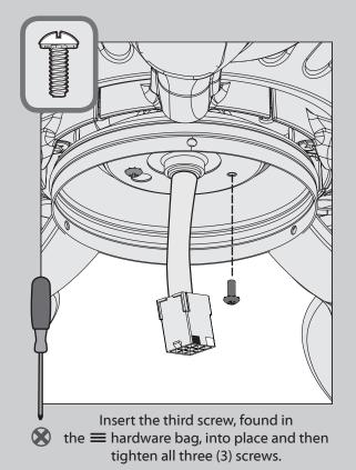
Make sure the upper switch housing is securely attached to the mounting plate. Failure to properly secure all 3 assembly screws could result in the switch housing fixture falling. Light Kit
