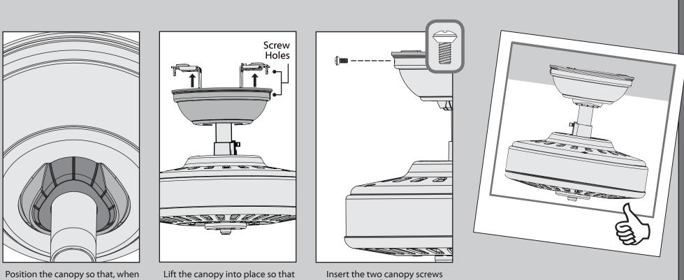
lifted into place, the canopy fits into the hanging bracket as shown.
