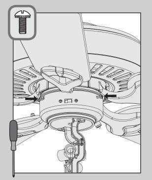
Install the third switch housing screw. Tighten all three screws securely.
