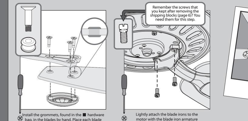
bag, in the blades by hand. Place each blade between a blade iron and medallion. Install three blade screws, found in the ▲ hardware bag, to attach the medallion to the blade iron. Repeat for all blades. Lightly attach the blade irons to the motor with the blade iron armature screws, then securely tighten after both screws are attached.
