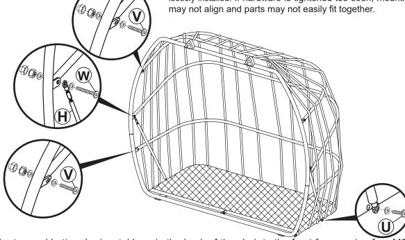
Loosely secure the top and bottom horizontal bars in the back of the chair to the front frame using four M6x22mm Bolt Sets (V).
