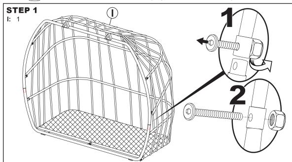
Locate and remove the two M6x35mm bolt sets from the frame of the chair, as shown.
