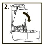
Unsnap and rotate screw cover plate downward to gain access to screw mounting holes.
