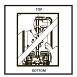
For proper dispenser tape adhesion: Press firmly all around backplate as shown in figure for 30 seconds. For maximum adhesion, do not load refill for 24 hours.
