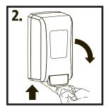
Press button on bottom of dispenser to open cover. Alternatively, use separate key tab to unlock cover.
