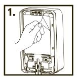
Peel paper off of installation tape and press dispenser firmly into position.
