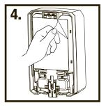
Peel paper off of installation tape and press dispenser firmly into position.
