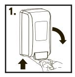
Press button on bottom of dispenser to open cover. Alternatively, use separate key tab to unlock cover.
