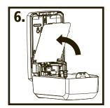
Rotate screw cover plate upward to hide screw mounting holes.
