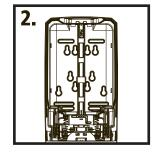
**2a.** Using Back Plate as template, mark and drill center holes in wall using 1/4" (6.3 mm) spiral masonry drill bit or 1/4" (6.3 mm) wood drill bit
