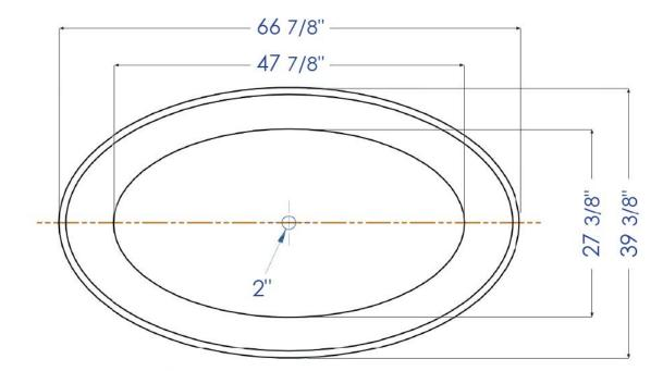
Please Note; Due to thermal expansion and contraction, the total dimension of the tub will have +-2% error, these dimensions are for reference only.
