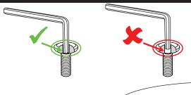
**Tip:** Always fully insert the hex key inside the designated notch of the bolt. If the hex key is not entirely inside the notch, the hex key could slip out, causing damage to the bolt head. In addition, repeated hex key slipping will cause the notch to become rounded, making it difficult or impossible to tighten the bolt.
