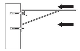
4 Place the sink in position against the wall. Locating sink onto the racks. Seal the rear of the sink from bottom. and level the top. Also Seal the rear of the backsplash onto the wall.
