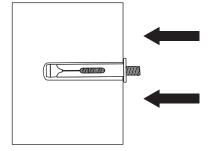
Measure the distance between the center of each mounting hole on the back of the racks. Use this measurement to draw 4 marks onto the wall in the desired mounting location. Use a level to make sure the marks are level with the floor. Drill 4 holes according to the marks using a 8 mm masonry drill bit to a depth of 55 mm.
