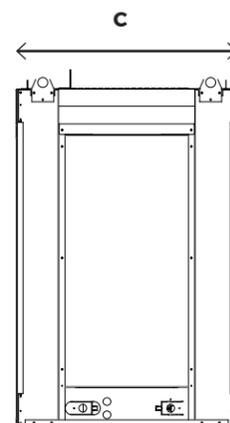
\*Finishing flange depth (The finishing flange defines the perimeter of the fireplace opening). Framing or finishing materials must NEVER encroach inside the finishing flange.
