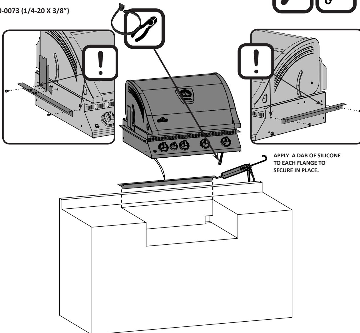
APPLY A DAB OF SILICONE TO EACH FLANGE TO SECURE IN PLACE.
