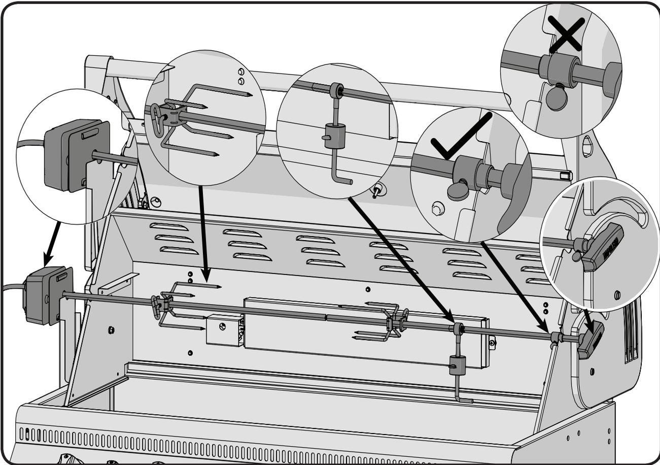
Ensure stop bushing is tightened on the inside of hood casting.
