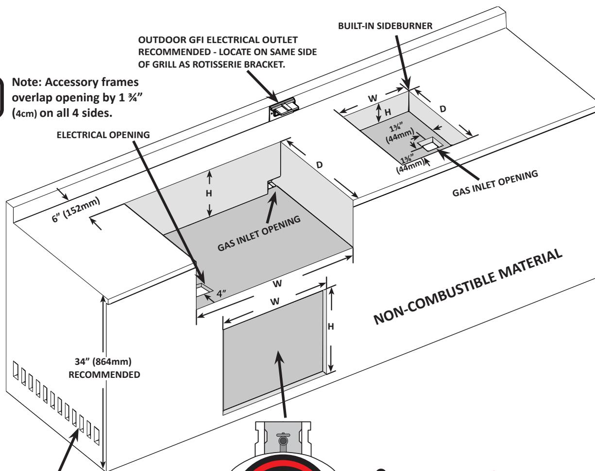
MINIMUM 10 SQ IN (65cm<sup>2</sup>) OF VENTILATION REQUIRED ON EACH END OF CABINET
