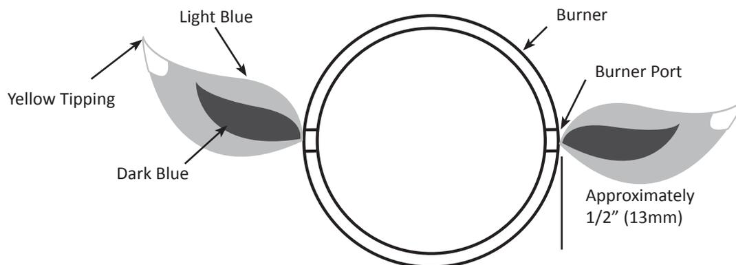
**Tube Burner:** The burners are made from heavy wall 304 stainless steel, but extreme heat and a corrosive environment can cause surface corrosion to occur. This can be removed with a brass wire brush.
