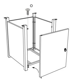
Step3. Hang the bottom (H) of the door plate on the round bracket. Top with 1PC screw(O)lock.
