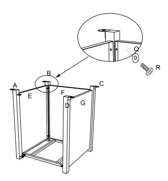
Step2. Connect panel (E,F,G)with table legs(A,B,C,D) by 12pcs screws (R) and 12pcs M6 washers(Q).
