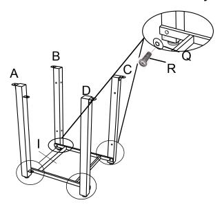
Step1.Connect the tank holder/base (I) With table Lets(A/B/C/D) by 4pcs screws (R)and 4pcs M6 washers(Q).
