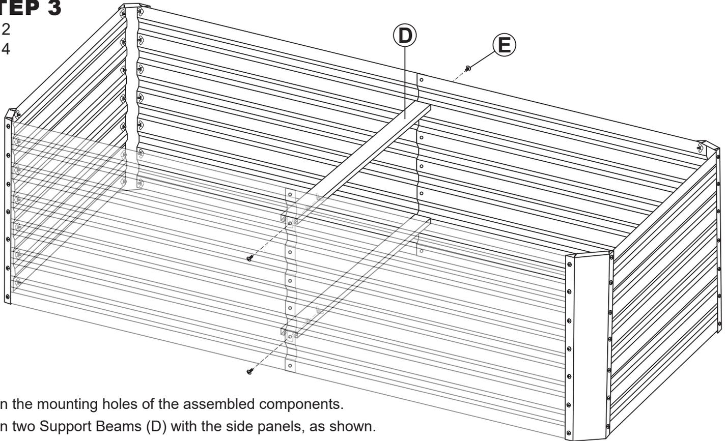
Align the mounting holes of the assembled components.
