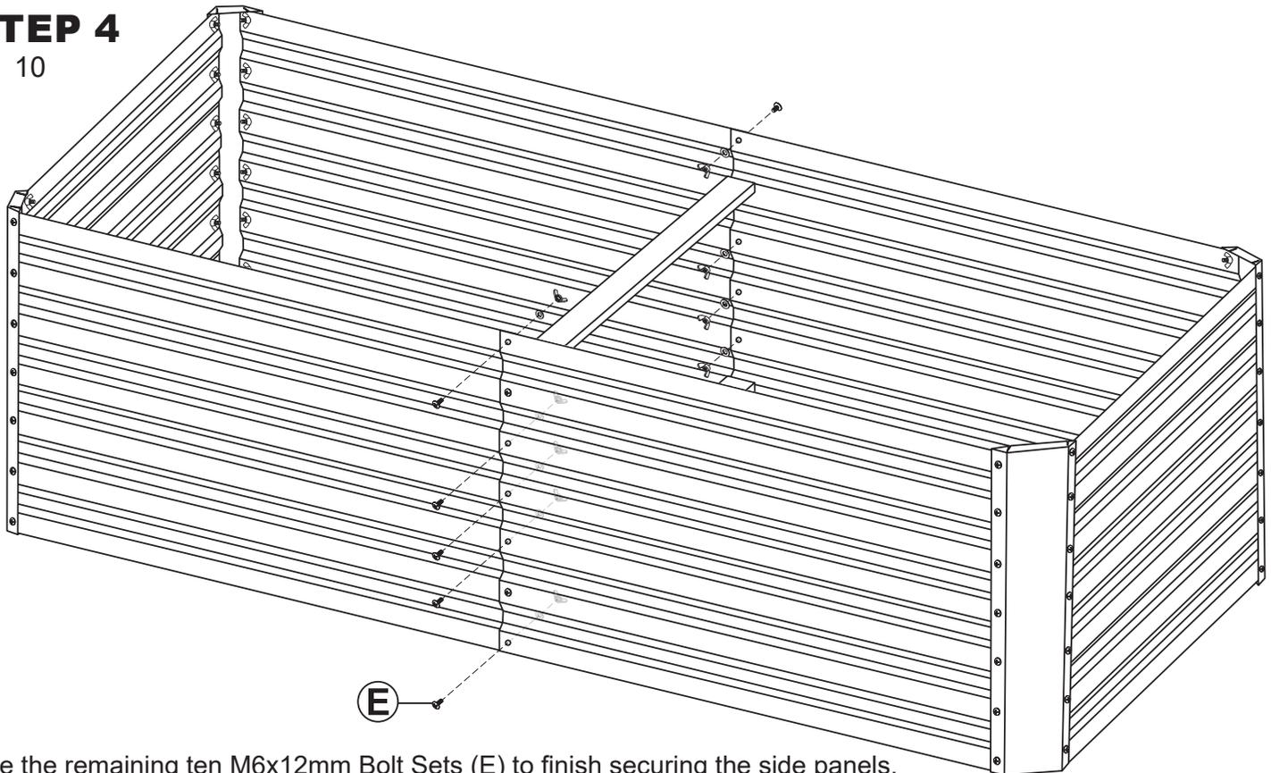
Use the remaining ten M6x12mm Bolt Sets (E) to finish securing the side panels.
