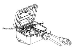
5. Secure the latch-on cover in the closed position and remove the clear protective mask on the front label of the device.
