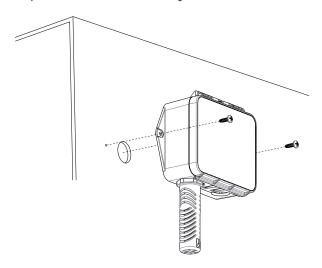
2. Ensure the probes are installed on the wall with no obstruction to airflow around the probe.
