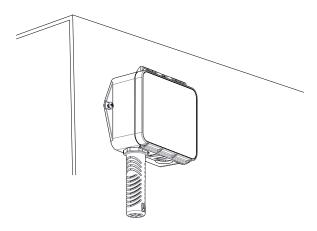
3. Release the latch on the lid to access the DIP switches and terminal block.
