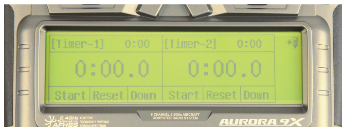
Touch the timer display on the home screen and it automatically reverts to this large easy-read layout.
