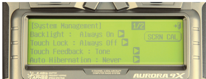
System Management is where you can adjust certain aspects of the transmitter's operation (see text for details).
