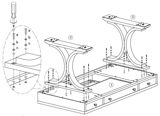
Step 1 : Put (A) upside-down on a clear soft surface to avoid damaging partsduring assembly.
