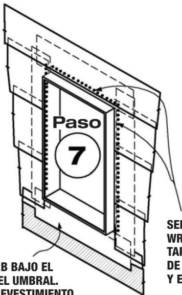
Figura 8 Instale WRB and seal around perimeter.
