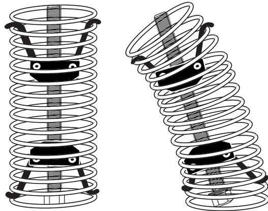
This tool is designed to handle springs up to 5-5/8 in. outside diameter and wire diameter of a maximum of 3/4 in.
