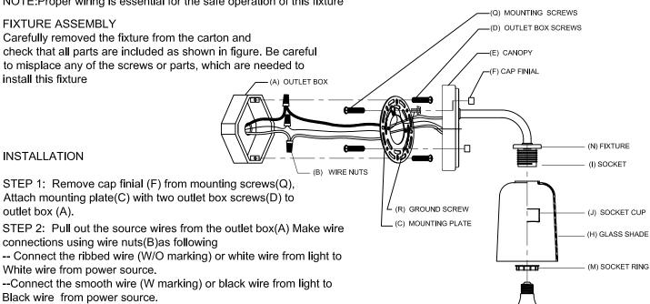
Carefully tuck the wires back into the outlet box.
