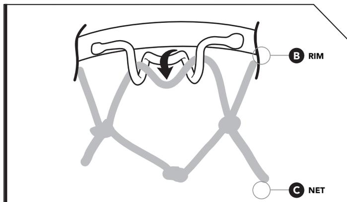
Attach the Net (C) to the Rim (B) by looping the long end of the Net over the metal loops.
