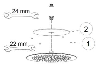
Put the felt covers (1) and the protection gasket (2) supplied on the upper shower head surface. Then, screw the kit to the shower head using a 24 mm wrench and a 22 mm wrench. The gasket (2) does not penetrate dust and/or air inside the cavity between the ceiling and the false ceiling as well as makes soundproof the area. The felt covers (1) protect the false ceiling from any possible scratches during the screwing process.
