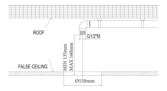
Run a pipe to the ceiling with G1/2"M outlet for the showerhead and prepare a false ceiling that must be at a distance between 135 mm and 160 mm.
