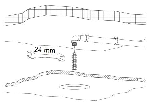
Then, screw hermetically the threaded connection using a 24 mm wrench together with hemp or similar materials.
