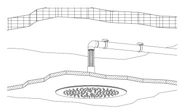
When the installation is completed, make sure that the shower head is perfectly stick to the false ceiling. This installation is the ideal solution for shower heads of huge dimensions and for any shower head with G 1/2 swivel.
