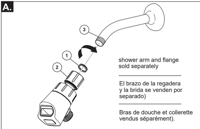
**A.** Verify there is a gasket (1) in hand shower mount (2). Hand tighten the hand shower mount onto the existing shower arm (3) (shower arm and flange sold separately). Do not use tools. The use of tools may cause product failure and will void the warranty.
