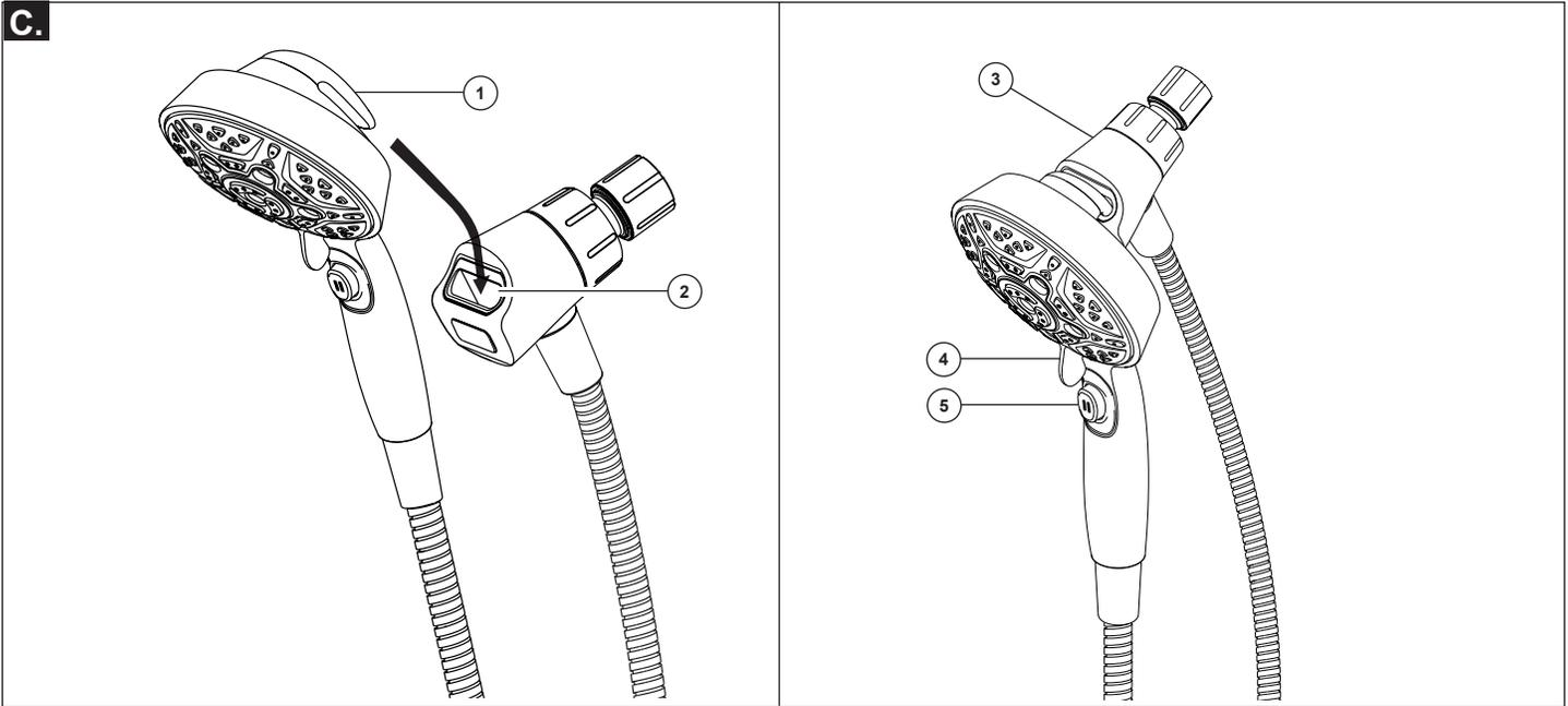
**C.** To dock the hand shower into the hand shower mount, insert the hook (1) on the handshower into the slot (2) of the hand shower mount. Pull the hand shower down into hand shower mount until the hook is fully seated (3). To undock, push the hand shower up out of the hand shower mount.
