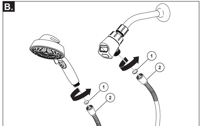
**B.** Verify there is a hose gasket (1) in the hose nut on each end of the hose (2). Connect one end of the hose to the hand shower mount and the other end to the handshower. All connections should be able to be made by hand tightening. Do not use tools. The use of tools may cause product failure and will void the warranty.
