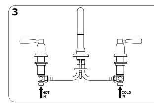
Connect and tighten the flexible hoses.
