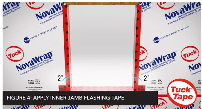
FIGURE 4: APPLY INNER JAMB FLASHING TAPE
