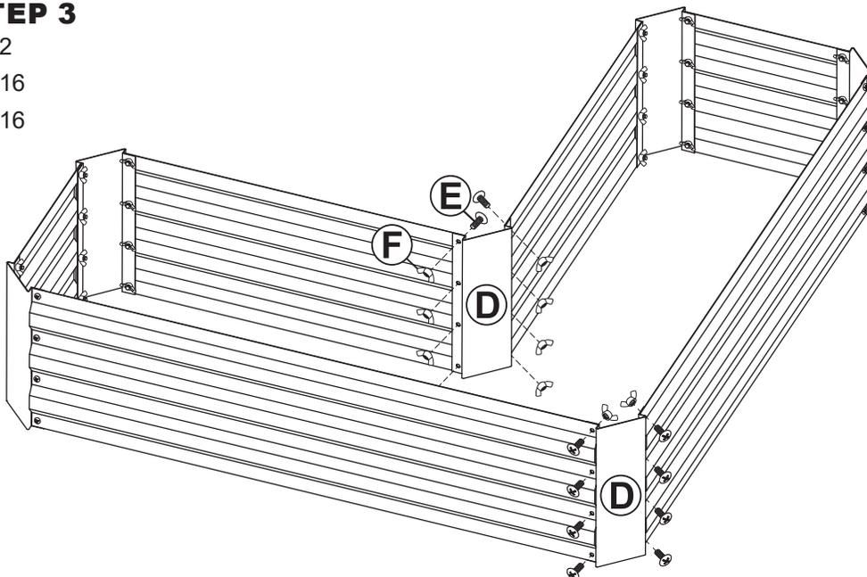
Loosely connect the long panels using one Corner (D), eight bolts and wing nuts.
