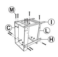
Align Leg Panel (I) with Planter Box (C) and Shelf (L). Loosely fasten using six Bolt Sets (M).
