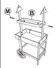
Firmly secure Tray (B) to the inside of the support posts using two Bolt Sets (M), as shown.
