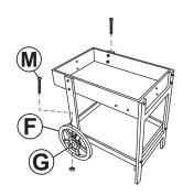
Slide Axle (G) through the mounting holes on the bottom of the front legs.
