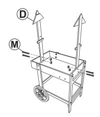
Ensuring the shelf supports are facing inward, loosely fasten two Support Posts (D) to the inside of the planter box using four Bolt Sets (M).
