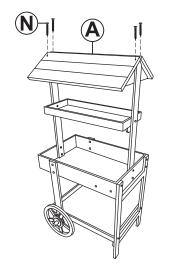
Place Roof (A) onto the support posts.
