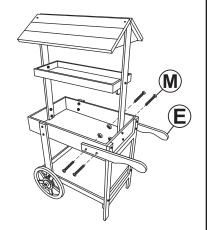
Align two Handles (E) with the planter box and secure using four Bolt Sets (M).
