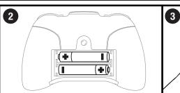
**2.** Install new batteries as shown in the polarity diagram (+/-) inside the battery compartment.
