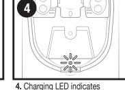
charging. Solid ON for charging and OFF when fully charged.
