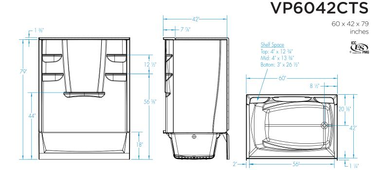
FEATURES Dimensional Tolerance ± 3/8". Dimensions needed for site preparation should be measured from the unit. Manufacturer assumes no responsibility for preparatory work.
