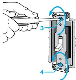
Disconnect all three wires\* from the switch.
