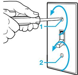
Remove the switch and pull it away from the wall.
