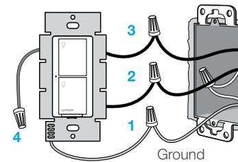
1 Connect the bare copper (or green) "ground" wire from the wallbox to the green wire on the switch using a wire connector.
