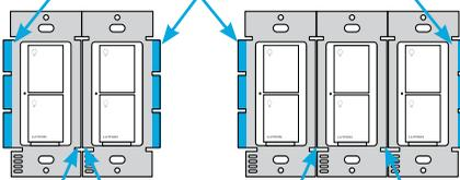
Each switch has inside side sections removed. Switch at middle has all side sections removed.
