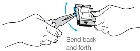
**Do not** remove outside side sections on switches at the end of gang.
