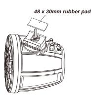
Place a supplied rubber (48 x 30 mm) pad on the metal base of the mounting band to prevent abrasion and secure clamping.
