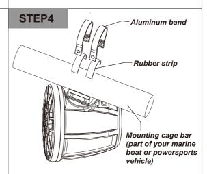
Place two supplied rubber strips around the cage bar to prevent abrasion and secure clamping. Then push two supplied aluminum bands over the cage bar, and align the aluminum bands with the metal base on the speakers.
