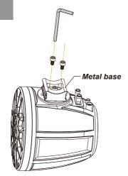
To adjust the mounting angle, loosen the metal base of the mounting band by unbolting the two screws.
