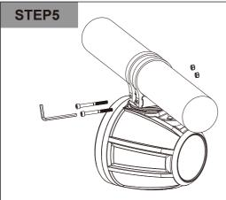
As illustrated, secure the aluminum bands to the metal base using a pair of M6 x 60mm screws, M6 flat washers, and M6 locknuts. The locknuts must be installed into the hex shaped recess on one end of each aluminum band.
