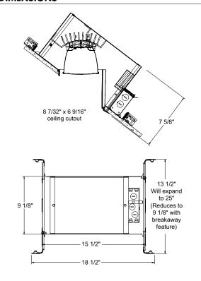
Mounting Frame 22-gauge die-formed galvanized steel mounting frame • Rough-in section (junction box, mounting frame, housing and bar hangers) fully assembled for ease of installation.
