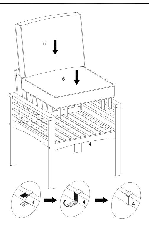
Put parts (5,6) into part (4) ,then tighten Velcro to part (4) as per diagram.
