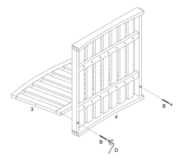
Using screw (B) attach part (4) to part (3) with hex key (D) as per diagram.
