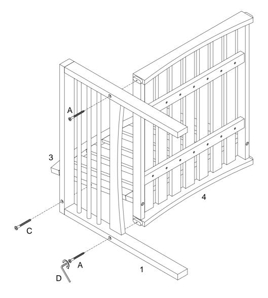
Using screw (A) attach part (1) to part (4) ,bolt (C) attach part (1) to part (3) with hex key (D) as per diagram.
