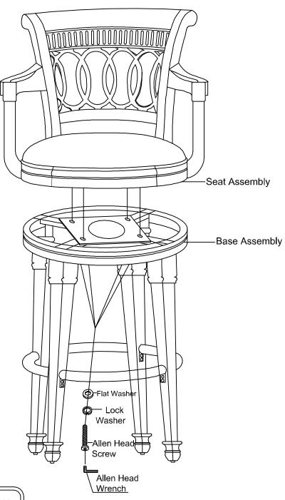
Attach the Seat Assembly to the Base Assembly with hardware as shown.
