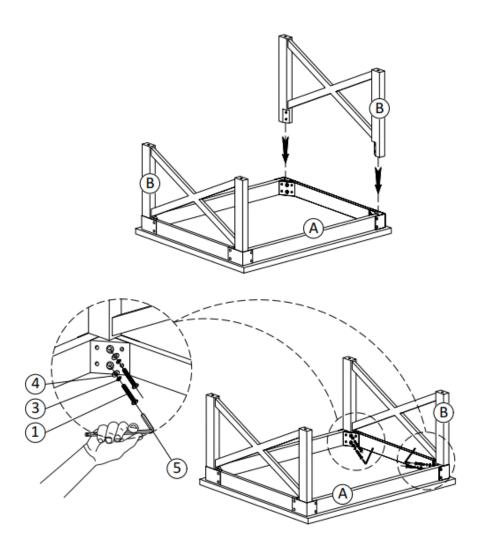
I. Repeat Step # I to attach second Side B to Top A.
