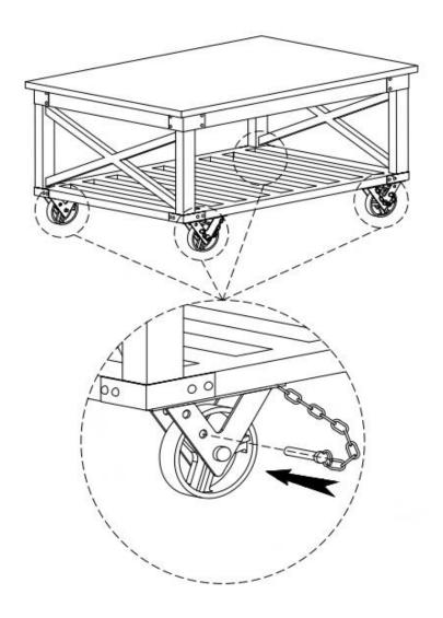
NOTE: Insert the pin in the Caster Wheels  $\bigcirc$  to lock in place.
