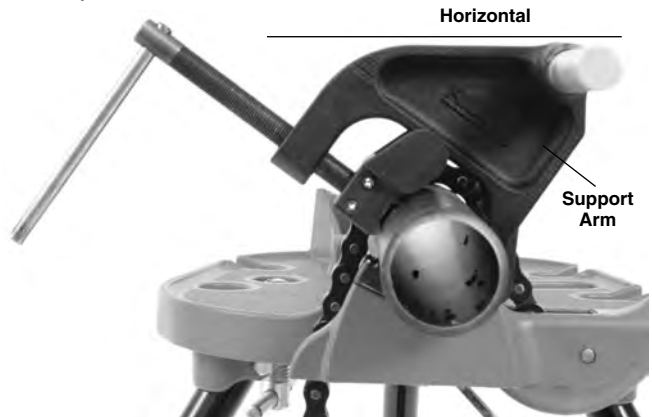
Figure 11A – Positioning the Support Arm
