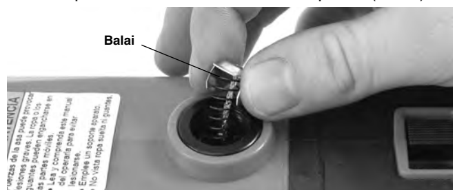
Figure 18 – Installation des balais
