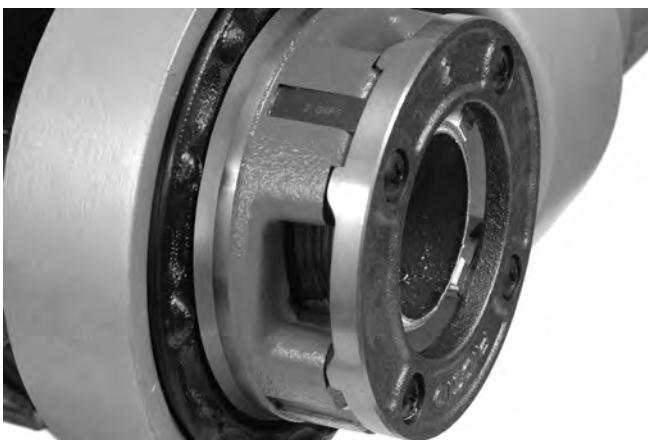
Figure 15 – Pipe Even with Edge of Dies
