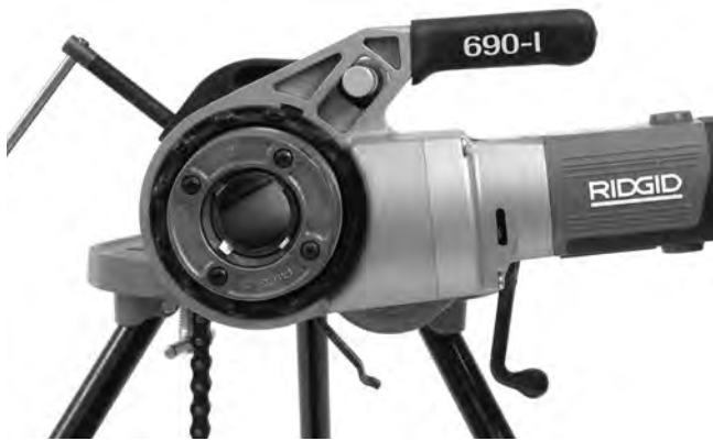
Figure 12 – Proper Orientation of the Power Drive
