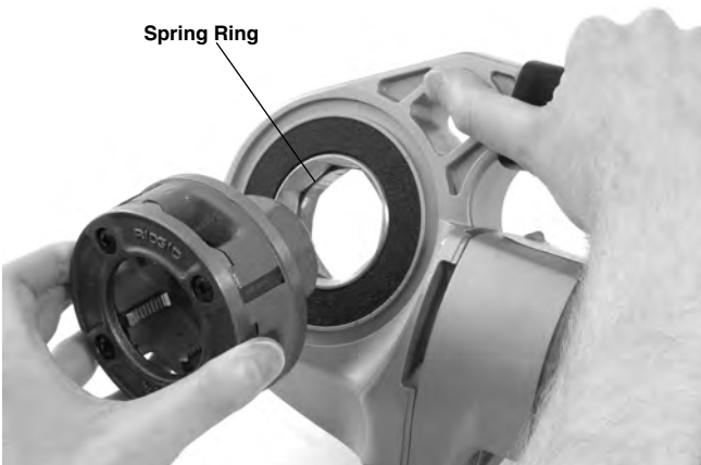
Figure 9 – Installing Die Heads into 600-I Power Drive
