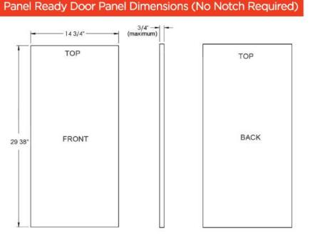
If making the panel 29 3/8", no notch (detail A,B) is required.
