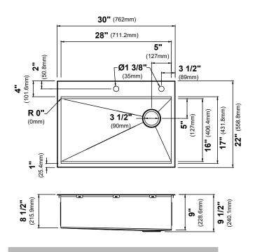
Model #: KWT310-30 Sink Dimensions: 30" x 22" x 9" Min Cabinet Size: 33"
